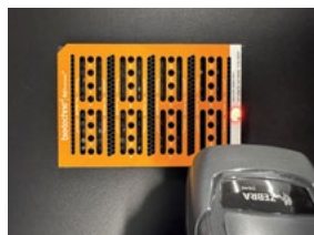
3. Scanning cartridge barcode for confirmation (optional).
