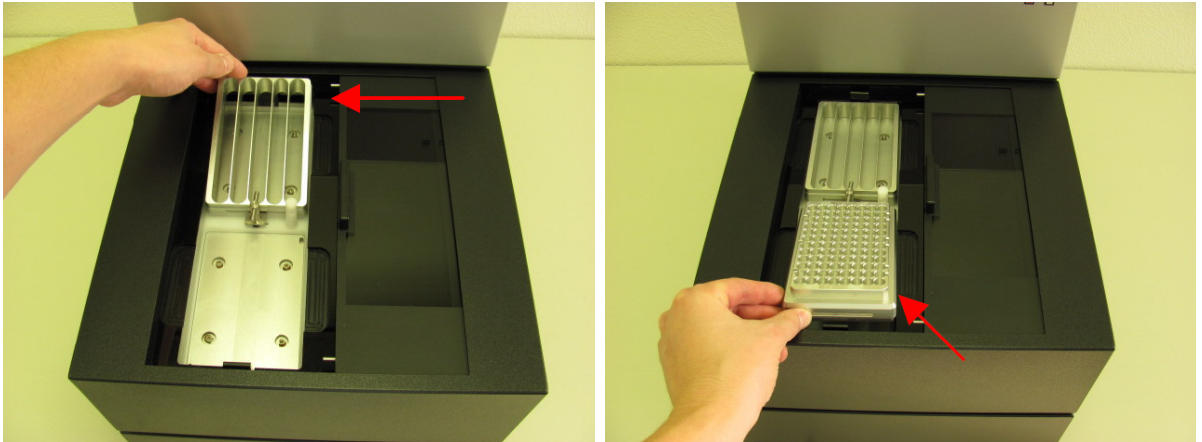
Figure 4-15: Inserting vial adapter in buffer tray (left) and adapter in sample tray (right) - 96-well plate adapter shown.
