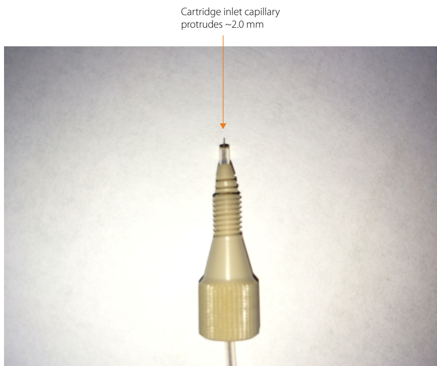
Figure 6-11: Cartridge inlet capillary approximately 2.0 mm past the cartridge inlet sleeve.
