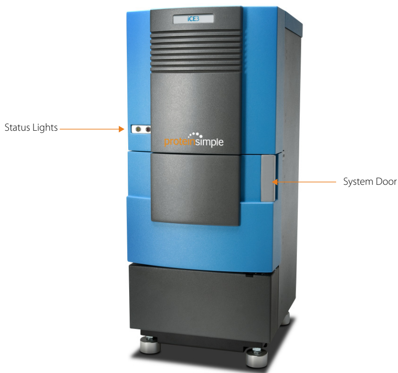
Figure 4-1: iCE3 instrument external components.
