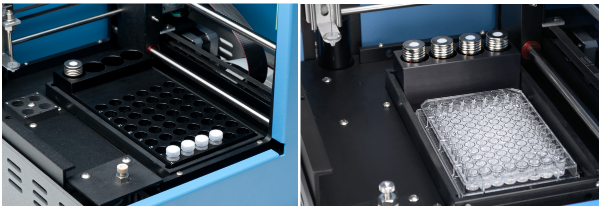
Figure 4-30: Alcott 720NV autosampler with 48/4 tray (left) and 96/4 tray (right).
