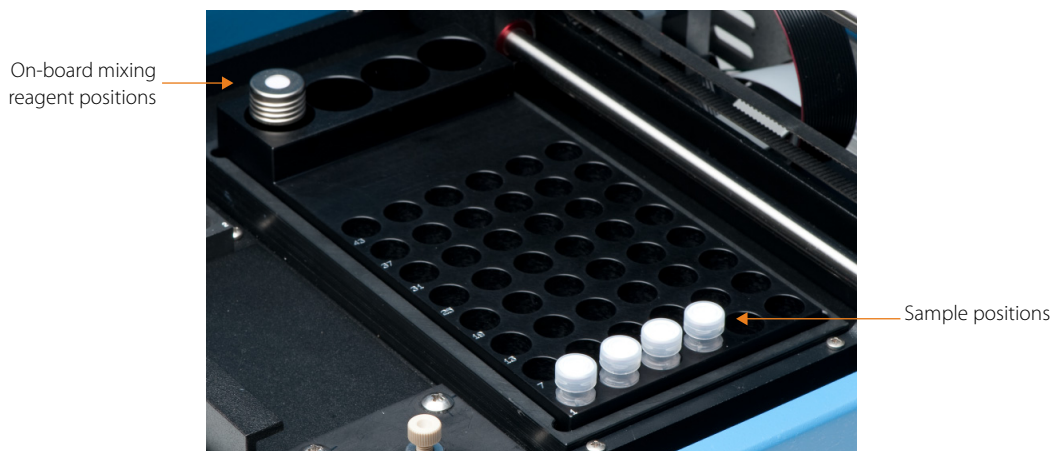
Figure 4-32: On-board mixing reagents and sample vial positions (48/4 tray shown).
