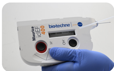
Figure 2. Cleaning the cartridge optical window from the side.
