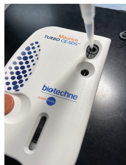
FIGURE 2. Filling the Top Chamber with Separation Matrix.
