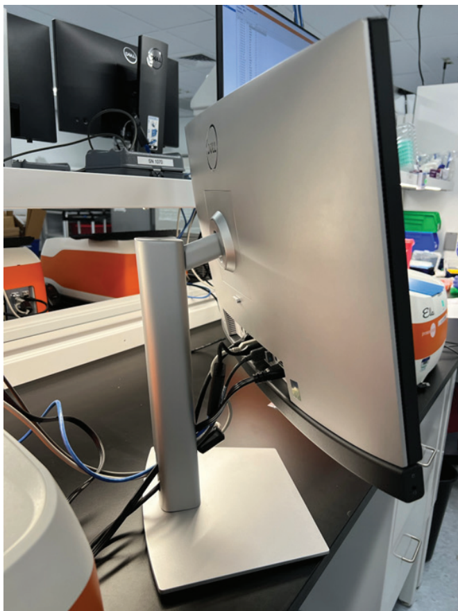
Figure 1-5: Back and front views showing cables from the PC directed through the hole in the monitor stand.
