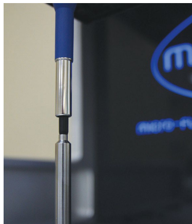
Figure 8-3: Bot I pipette unit positioned over calibration pin.
