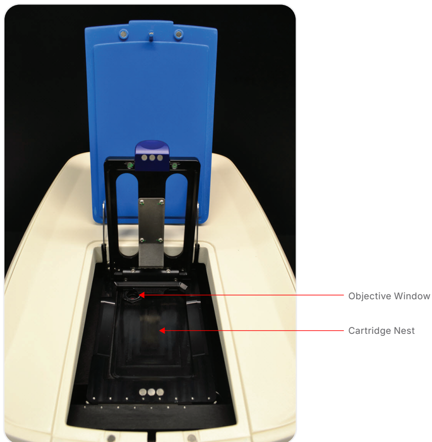
FIGURE 5-9. Cartridge Nest and Objective Window
