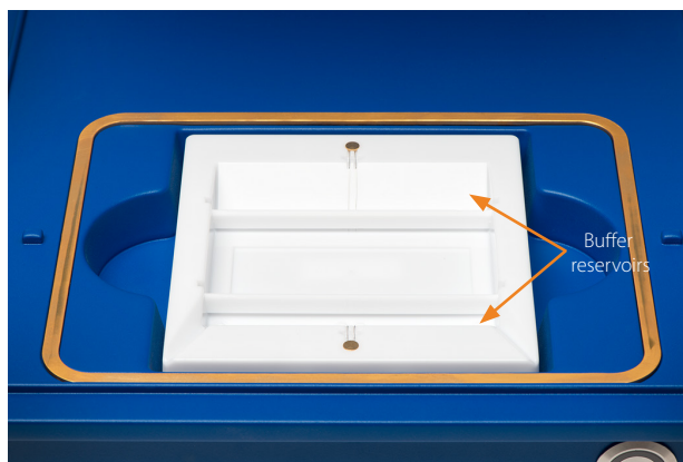
Figure 5-13: Lysis/Run Buffer should be added to the upper or lower reservoir of the electrophoresis cell. It will spread to cover the scWest chip. Reservoirs are indicated by arrows.
